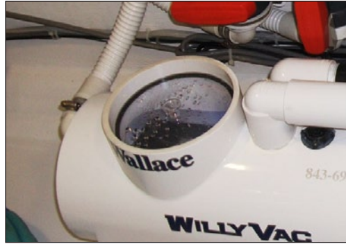
Figure 11: Strainer Basket and Plexiglas Lid
